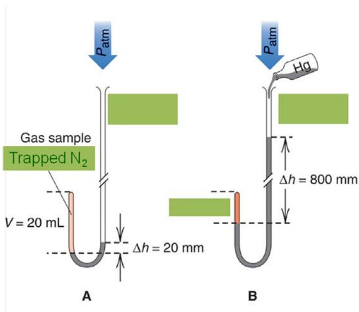
(a) (4 pts) What is the pressure of the trapped  $N_2$  gas in the initial state (that is, before more mercury was added as shown in A) and the final state (after adding more mercury as shown in B) (2 pt for each correct answer and otherwise 0 pt)?
