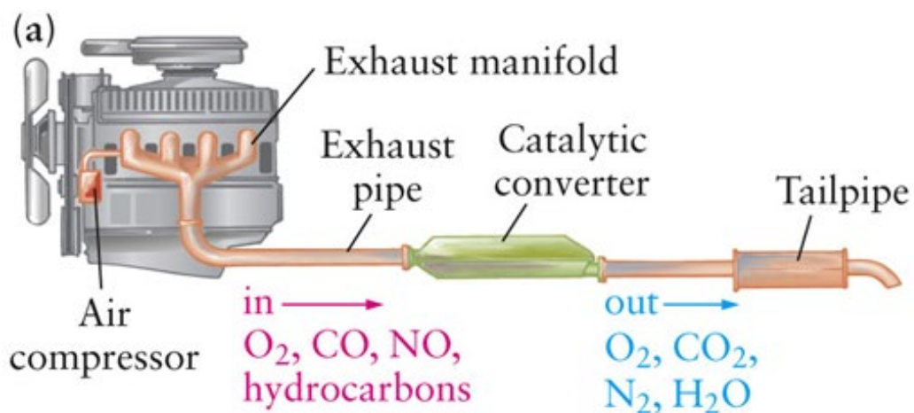
Fig. 18.21 (a) A catalytic converter used to reduce car pollution and (b) its inside.
