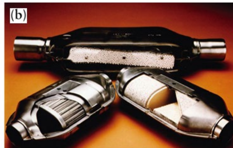
Fig. 18.21 (a) A catalytic converter used to reduce car pollution and (b) its inside.
