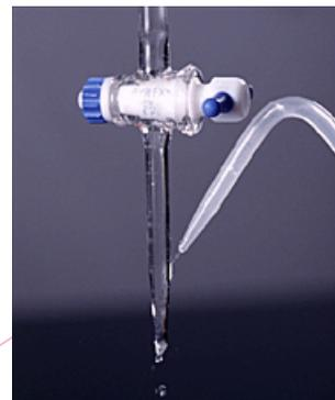
3. Using the procedure described above for adding solutions to the buret, fill it to a level just above 0.00 mL. Drain the buret to just under 0.00 mL. This will properly form the meniscus. **DO NOT ATTEMPT TO ADJUST THE MENISCUS TO EXACTLY 0.00 mL. THIS IS AN INCREDIBLE WASTE OF TIME.**
