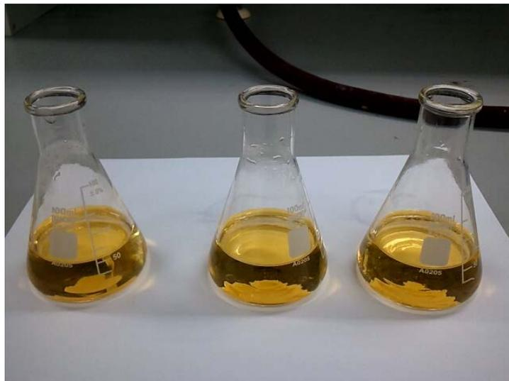
Dispense the HCl solution from the buret, swirling the Erlenmeyer flask during the addition. Carefully add additional HCl titrant until the endpoint is reached and the color persists for 30 seconds. (a color change caused by the addition of one additional drop of the HCl solution from the buret) Stop the HCl titrant. After 10-15 seconds, record the volume of HCl in the buret.
